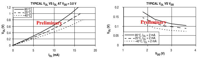
Table 14. Typical Low-Side Driver (Sink) Characteristics (LCD/GPIO pins)— Low Drive (PTxDSn = 0)
