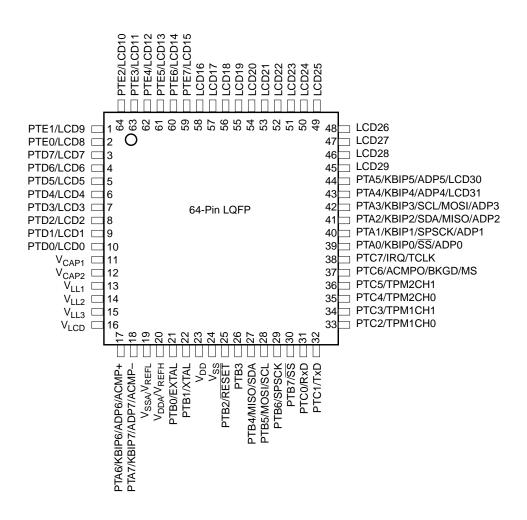
Note: V<sub>REFH</sub>/V<sub>REFL</sub> are internally connected to V<sub>DDA</sub>/V<sub>SSA</sub>.
