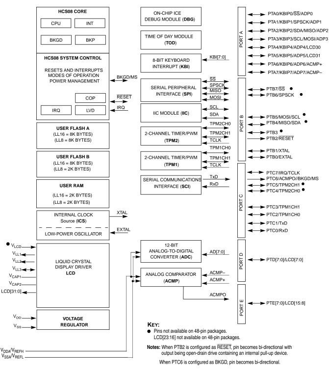
Figure 1. MC9S08LL16 Series Block Diagram
