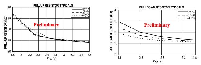
Table 9. All I/O Pullup and Pulldown Typical Resistor Values (V<sub>DD</sub> = 3.0 V)
