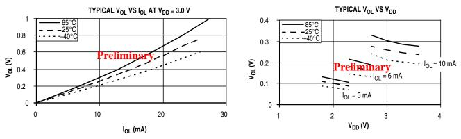
Table 15. Typical Low-Side Driver (Sink) Characteristics(LCD/GPIO pins) — High Drive (PTxDSn = 1)
