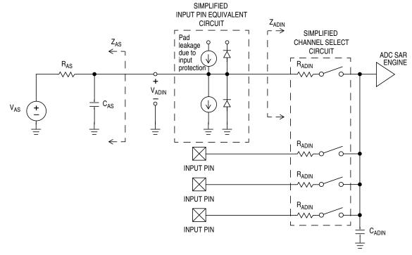
Figure 17. ADC Input Impedance Equivalency Diagram
