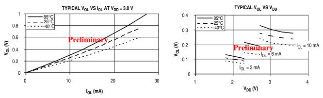
Table 11. Typical Low-Side Driver (Sink) Characteristics(Non LCD pins) — High Drive (PTxDSn = 1)
