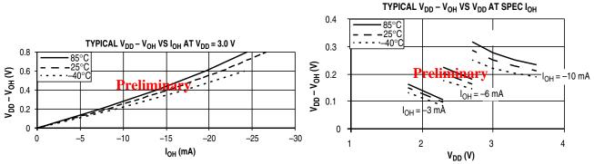
Table 17. Typical High-Side (Source) Characteristics(LCD/GPIO pins) — High Drive (PTxDSn = 1)
