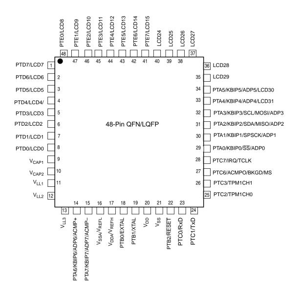
Note:  $V_{REFH}/V_{REFL}$  are internally connected to  $V_{DDA}/V_{SSA}$
