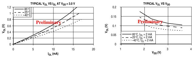
Table 10. Typical Low-Side Driver (Sink) Characteristics (Non LCD pins)— Low Drive (PTxDSn = 0)
